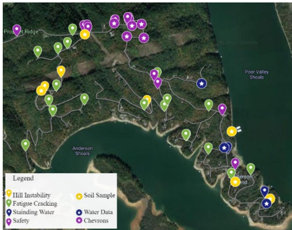
Figure 5: Inventory of Damages
